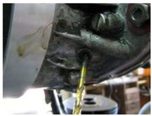
Introduce (carefully) a 3mm dia and 100 long metal pin (say a drill 3mm with its non spiraled end) into the timing opening.
