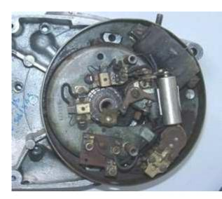
Disconnect the cables from your old generator and remove it. Unscrew the old stator and take it off the engine. Pull the rotor off, you will need a puller screw for this.
