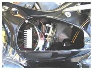
Fasten the regulator/rectifier unit, the relay and the ignition coil on a convenient place, maybe in the side pocket.
