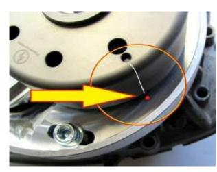
Have a look at the new rotor. You will find on its circumference a small pressed in line. Then have a look at the ground plate. There you will find a red point marker. These are ignition markings. They have to align at the point of ignition.
