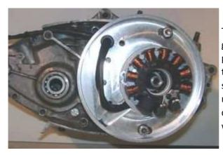
Take off the cover holder plate from your new generator. Place the preassembled unit (ground plate/stator) at the ignition system mounting of the crank case. Screw it tight with both M8 screws. You should set the screws in the center of mounting holes, so you have the possibility for correction. Please don't forget to use the washers.
