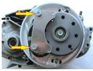
Replace now the cover holder plate on the ground plate. You have to put the two M8x60 screws through the holes in the cover holder plate and the two spacers. Then screw it tight on the ground plate.
