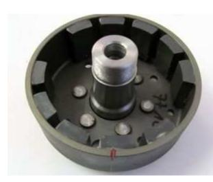
Take a look at the new rotor. You will find on its circumference a small lasered in line which is continued at the top of the side wall in red. That is an ignition marking.
