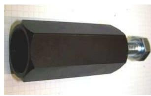
To disengage your new rotor again, you will need to use the <u>supplied</u> puller M27x1.25 (part-no.: 72 98 799 99).
