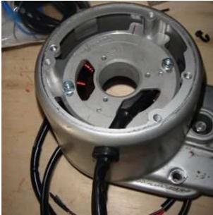
Remains to make some way to lead the wire out of the cover.
