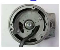
generator/electronic ignition for <u>Suzuki T125</u> (not for GT125!)
