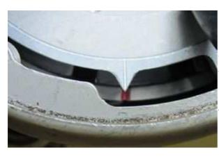
With crank still in ignition position check whether the rotor marking and the stator indicating pin align.
