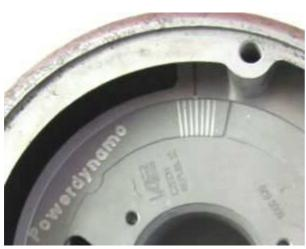
Now, to fine tune, you may loosen a little (!) the 2 holder screws you have at the bottom and turn the base (magnets will pull against you) until the 2 markings align.
