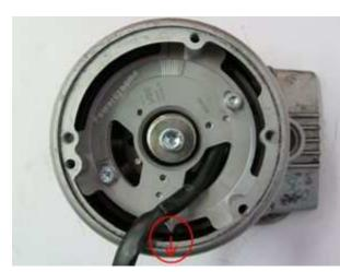
As the screws are 120 degrees apart and hence permit 3 different settings of the stator unit, make sure to get correct position of the stator. The correct position is when the indicator pin at the base plate (encircled in picture) points vertically to the ground as shown here.
