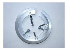
Place the adapter onto the engine. The wire opening of the adapter will show to about 2 o'clock, Screw the adapter down with the 2 countersunk screws M4x15 (the countersunk holes).
