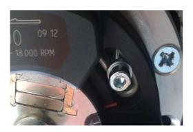
To be able to use the long holes to adapt timing, fix stator in middle position of those long holes.
