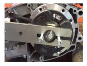
To help turning the rotor and to stabilize it during fastening, use the supplied tool as shown here in the picture.
