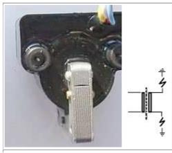
In our twin outlet coils both ends of the secondary go to spark plugs.
