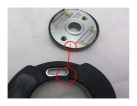
Set any of the 2 pistons into ignition position. In that crank position place the rotor onto the crank in such a way, that the small red marking on the rotor aligns with the red line on the inside of the stator. Take care not to change the set position of the crank during that operation.
