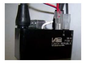
The wider 6.3mm pin to connect to the red/white wire brings the ignition voltage. The narrower, 4.2mm pin gets the impulse from the black wire.
