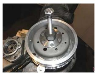
In that position, screw the rotor down with the provided screw M8x1 (place the washer there).
