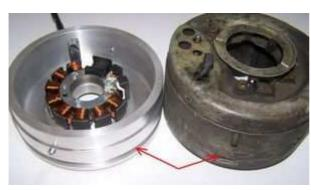
Have a look at the new stator unit. It has at the bottom some groove going all around the unit.
