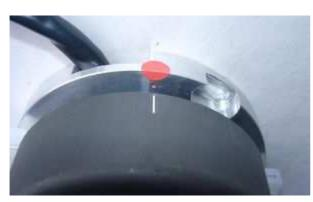
Before you screw the rotor down to the shaft, you will have to set ignition:
