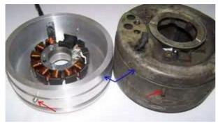
Remains to place the stock cover over the new unit and fasten it with the stock holder clamp.
