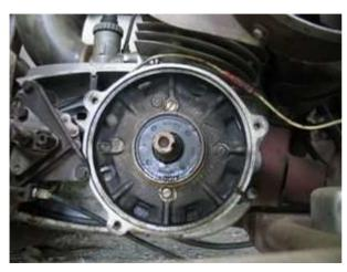
Place the stator unit onto the engine and fix it with the 3 stock clamps.
