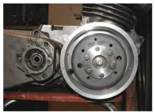
Place the rotor onto the shaft.
