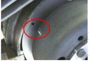
Bring the piston into ignition position. This is somewhat before top dead center (BTDC). Value is given either in mm or degrees BTDC. If you do not find any value try with 2.5mm and correct than later depending on tests.
