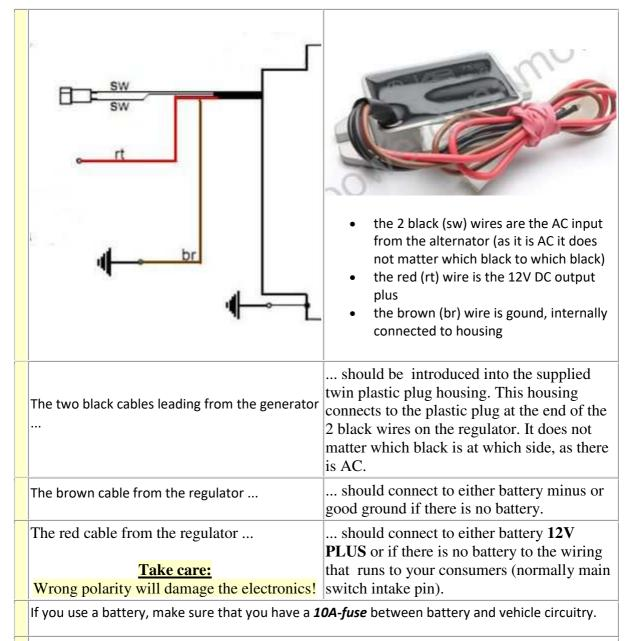
There is NO facility for a charge control light without battery this will not work anyway. The regulator has an inbuilt high potency condenser to smoothen voltage. This will make sure that your side indicators (flashers) and horn will work correctly even without battery.
