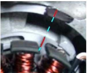
As the ignition marking on the base plate will not be visible once you have put the rotor, you will have to transpose it to some point further out.
