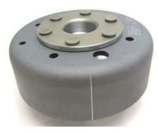
Have a look at the new rotor. You will find on its circumference a lased on (older rotor: pressed in) line. That is an ignition marking too. It is durable, but not well visible, so better highlighten it with some marker pen.
