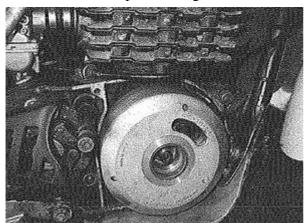
Pull the stock rotor from the crank (you will need a puller for this), unscrew the old stator and take it off the engine.
