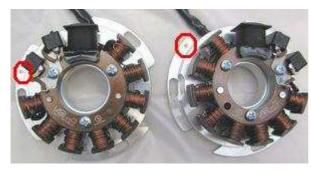
Have a look at the new stator unit. You will find there left from the larger black coil a small red marking. This is an ignition marking for timing.
