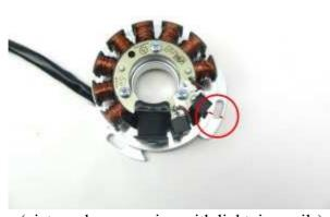
(picture shows version with lightning coils)
