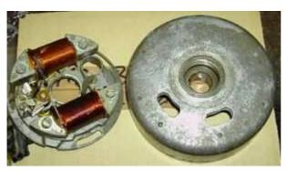
Disconnect the wires from the old magneto. Pull all wires out of the engine housing.
