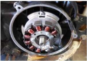
Put the stator unit onto the motor. Centre it upon the 3 mount holes and screw it down with the 3 screws M5. The cable shows in direction of the cable exit of the casing.
