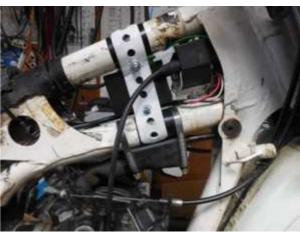
Before installing the advance unit, have a look at the small switches at the advance unit. They activate different characteristics. There are 4 switches.
