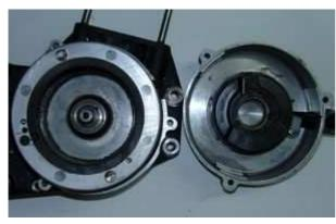
Unscrew the old stator and take it off the engine. Pull the rotor off, you will need a puller for this. Take the woodruff key from the crank. You will not need it any more. Please do not forget to do so, otherwise you will have trouble later on in the assembly.
