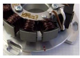
Take a look at the new stator unit. You will find there (next to the smaller black coils) a little red ignition marking. This marking is not visible if the new rotor is on its place. Therefor you have to transfer this marking onto the engine housing.
