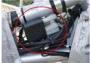
Here you see a suggestion of a customer how to mount the ignition coil and the control unit:
