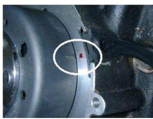
Take the spark plug out and bring the piston into TDC (the highest point, the piston should reach). Place the rotor loosely onto the crank, check that it may move freely above the statorbase and use it for moving the piston.
