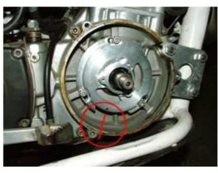
Now you can transfer please the stator's ignition marking onto the motor housing. Proceed carefully. The (imaginary) straight line from the center of the crankshaft must be extended beyond the existing ignition marking out.
