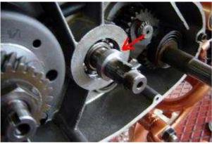
Replace the factory spacer ring under the primary gear with the thicker version supplied in the kit.
