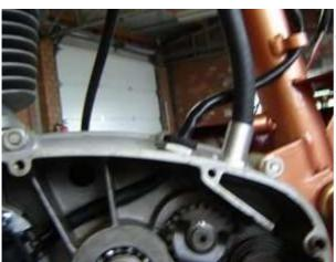
Usher the stator cable through the wire openings of the engine - from inside out.
