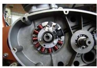
There should be no need to take the stator coil from its base. Should you however need to do so, take great care when setting it back. The stator has to snap in rather sharply. If it sets softly there, you have probably squeezed a wire underneath!
