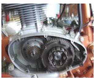
Place the clutch assembly onto the gearshaft.
