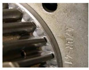
Check that the large clutch gear does not brush against the collar on the rotor (see picture). Eventually put the provided shim(s) (0.5/1.0mm) underneath the clutch.
