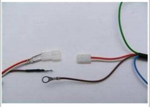
Look for the advance unit with its female plug and the two wires (red and white).
