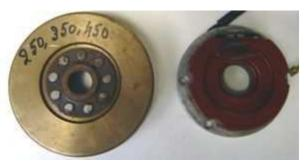
Unscrew the generator cover and take it off. Unscrew the stock magneto and take it off.
