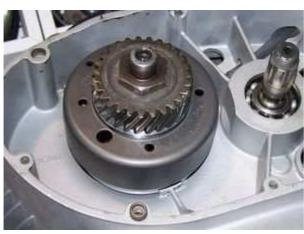
Now set the woodruff key back onto the crank shaft and place the primary gear on top of the rotor. Screw the rotor down as per original instructions.
