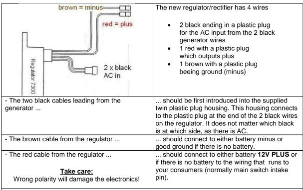
Make sure that you have a 15A-fuse between battery and vehicle circuitry.
