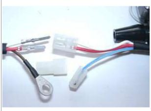
Look for the ignition coil with its female plug and the three wires (red and white).
