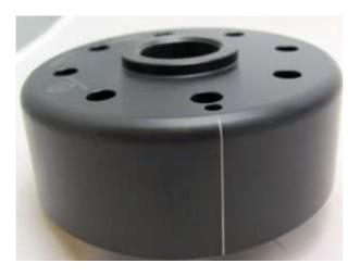
Have a look at the new rotor. You will find on its circumference equally some marking (a pressed or lasered in line).
