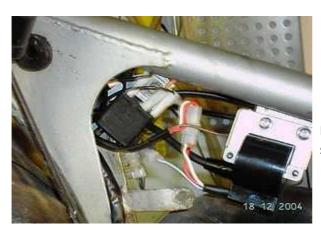
Fasten the regulator at some convenient spot on the frame.
