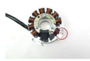
Place the pre-assembled stator unit onto the engine's magneto seat and screw it down there with the 3 screws M5. Lead the wire from the new generator through the wire opening of the engine upwards along the frame (or downwards).
