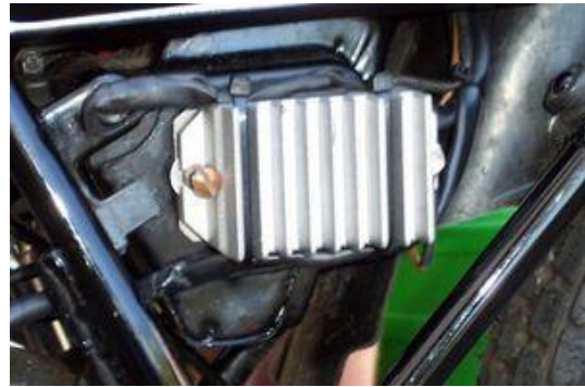
- Picture shows larger regulator as used in older installations. Now a smaller, but as effective regulator with additional inbuilt smoothing condenser is used
