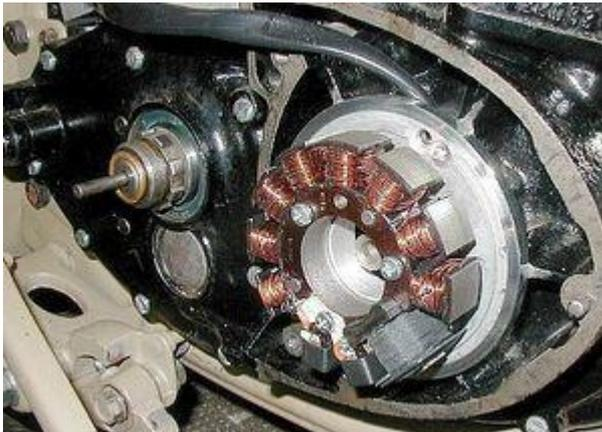
Once the plate is fixed, reset the stator coil onto it. Here make double sure not to pinch any wires underneath. As the coil sits quite low in the engine, this is difficult to see.
