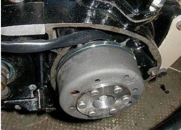
When the rotor is correctly installed, replace the spark plug. If you used the rear wheel to rotate the engine, change gears back to neutral.
