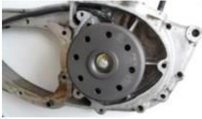
Magnet based generator with integrated fully electronic ignition. Output at 12V/150W DC. Solid state ignition with own power supply from within the system. Replaces old dynamo, points, condenser, ignition coils. No changes on engine casing needed.
