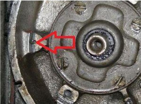
Take the small arresting pin off which was there to set the stock dynamo correctly. If you forget the new base plate will not sit correctly, leading possibly to severe stator/rotor damage.
