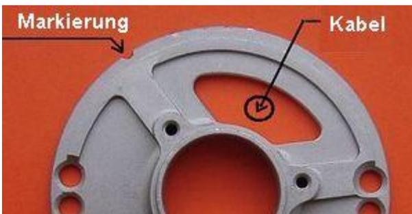
Take a look at the stator base plate (aluminium). You will find there, left from the cable passage ("Kabel"), a small notch ("Markierung") on the circumference.
