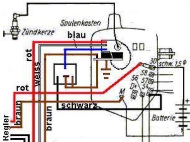
Connect the red, the white and the brown ground cable (from the new generator) and the blue cut-off cable to the new ignition coil.
