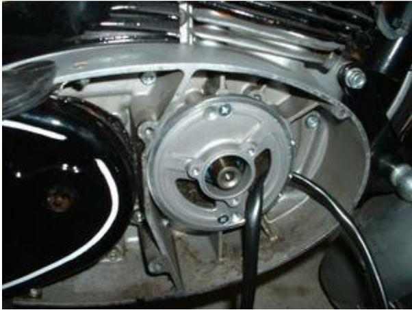
Remove the 3 fixing screws which hold the stator coil to its base. Now you can lift-off the coil a little away from the ground plate (ca. 1cm). So as the mounting holes on the ground plate become accessible. Don't damage the paint insulation!
