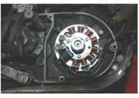
Now look at the rotor, on its outer perimeter you will find a small marking (a knurled line). Here in the picture highlighted white for better visibility.
