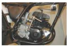
Magneto based ignition device with integrated fully electronic ignition dependent on speed. Light output 12 V/180 W DC. Contactless electronic ignition with its own power supply inside of the device. Replaces old dynamos, centrifugal regulators, breakers, ignition coil. (If the regulator is not required, the device can be delivered also without it!) No changes to the engine casing required!
