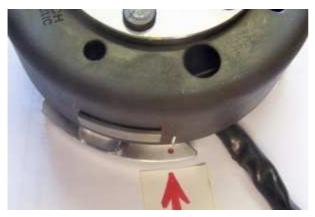
Remove the spark plug and move the piston to the "ignition point" position. (Or alternatively 2 mm from OT, anyway consult this in the motorcycle's instruction manual!) Because it is quite complicated due to the start lever, use the new rotor to rotate the crankshaft.
