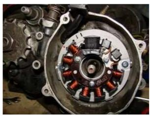
Place the preassembled unit (adapter plate/stator) at the ignition system mounting of the crank case.
