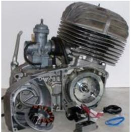
Generator/electronic ignition for: CZ 250cc moto-cross (typ 980) from Sidepipe (1968) to 1974, CZ 380cc (typ 981), early CZ 125 motocross up to 1974 and possibly (not confirmed) CZ500
