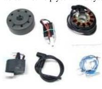
Magnet based generator with integrated fully electronic ignition. Output at 12V/100W DC. Solid state ignition with own power supply from within the system. Replaces old magneto, pickup, regulator and ignition coil.
