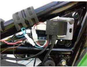
Fasten the new electronic rectifier/regulator and ignition coil at an convenient place. Before you fix the coil, screw in the high-tension cables. Lay the new generator cables along the frame (using the enclosed cable binders), in that way, that they finished close to the regulator resp. ignition coil. Take care that nothing's pinched.
