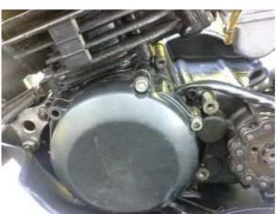
Place the engine cover back. Check that it does not interfere with anything.
