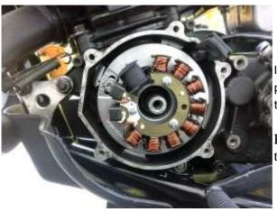
Insert the new base plate with the stator in the place of your old stator and fasten the plate with the two provided M5 screws.
