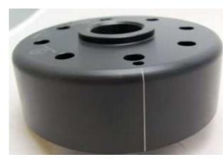
Take a look at the new rotor. You will find on its circumference a small pressed in line. That is an ignition marking. It is durable, but not well visible, so better highlighten it with some marker pen.
