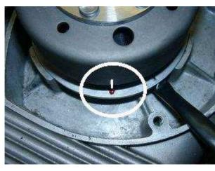
Take the spark plug out and bring the piston into top dead center position (TDC), that is the highest point the piston should reach. As this is difficult to do with the kick lever, place the new rotor onto the crankshaft (do not screw it down) and use it as a handle to turn the crank.
