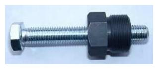
To pull the new rotor again, you need a puller M27x1,25 (part-no.: 99 99 799 00 -Not provided!-).
