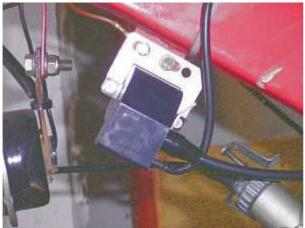
Fasten the new ignition coil at the same place, as the original. Leave one screw loose, you have to connect a ground cable here.
