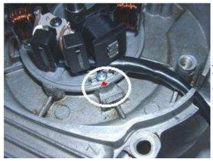
**Note:** Should you remove the stator completely from its base, take a note of its position there. A changed position would need an ignition mark shifted by 120°.
