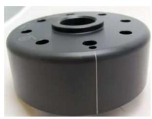
Have a look at the new rotor. You will find on its circumference a small pressed in line. That is an ignition marking as well. It is durable, but not well visible, so better highlighten it with some marker pen.
