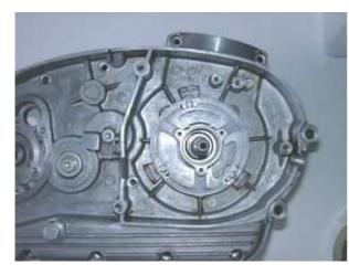
Unscrew the stator (3 screws M4) and take it off the ground plate.
