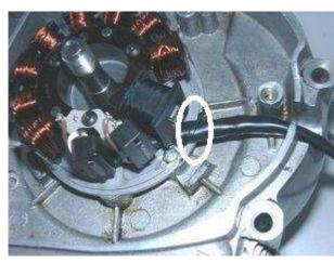
Put the stator coil back onto the plate. The stator has to snap in rather sharply. If it sets soft, you have probably jammed a wire underneath! Make sure that the inner opening of the stator unit slots evenly over the elevated fixing rim of the base plate - otherwise the coil will sit lopsided and will touch the rotor, damaging it.
