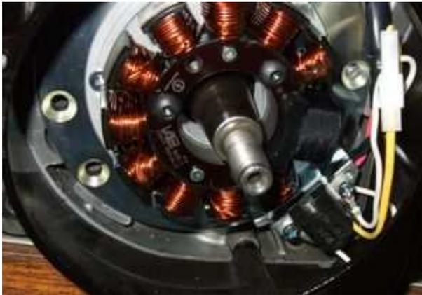
Place the stator unit onto the engine. Pickup module showing to about 5 o'clock
