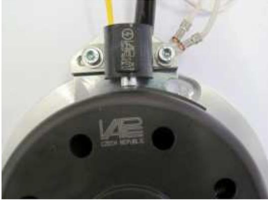
Ignition timing is done by setting the rotor in a certain position to the sensor.
