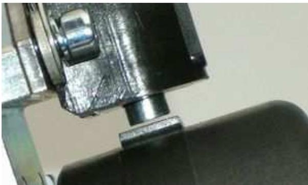
Check that the metal pin of the sensor runs about middle of the trigger sign on the rotor. The more it is outside, the harder starting is.
