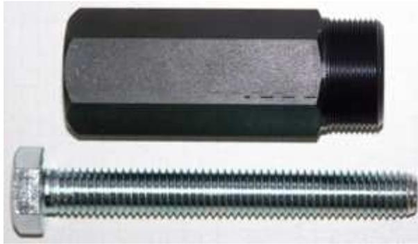
To disengage your new rotor again, only use the supplied long puller M27x1,25 (part-no.: 71 69 999 99).
