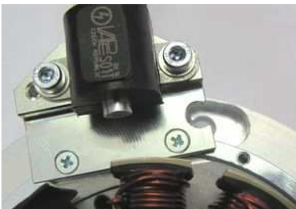
The stator assembly is fastened by 3 supplied socket head screws M6x12. As the one of them near the pickup is obscured by the pickup holder, the holder has been opened a little so that the allen key can be applied. There is no need to take the sensor (pickup) holder off.
