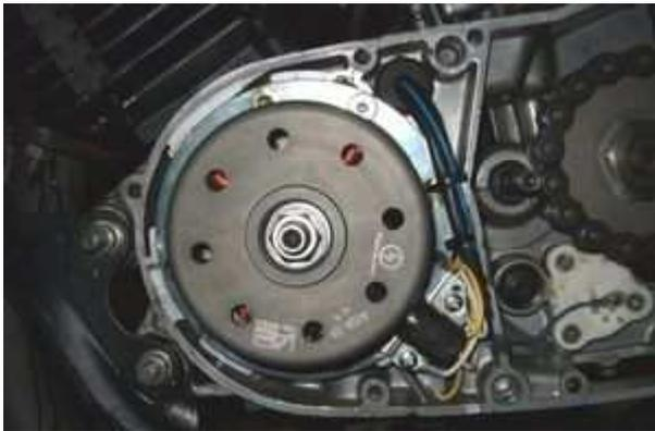
Tighten the rotor with the stock nut, not forgetting the supplied washer and bush as the threading is quite long. To undo the rotor use a puller M27x1,25. With that the work on the engine is finished. Put the spark plugs back.
