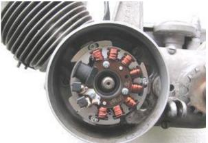
Place the pre-assembled stator unit onto the engine's magneto seat and screw it down there with the 3 screws M5.
