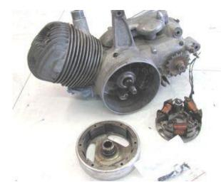
Disconnect the wires from the old magneto. Pull all wires out of the engine housing. Take the magneto off.
