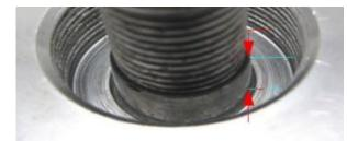
Before you set timing however check carefully that the rotor may turn freely above coil and plate.
