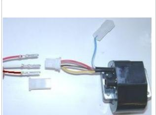
Look for the ignition coil with its female plug and the three wires (red, brown and yellow).
