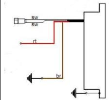
The new regulator/rectifier has 4 wires
