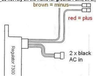
The new regulator/rectifier has 4 wires
