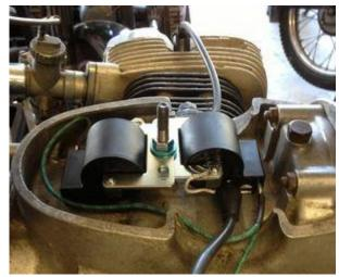
The system has **2 single ignition coils** (as the twin coil is too large to mount it under the top engine cover).
