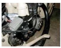
Magnet based generator with integrated fully electronic ignition. Output at 12V/100W DC. Solid state ignition with own power supply from within the system. Replaces old dynamo, points, centrifugal governor, ignition coils. No changes on engine casing needed. You may drive without a battery, if you want.
