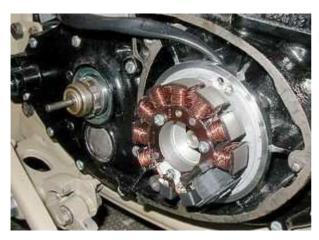
Once the plate is fixed, reset the stator coil onto it. Here make double sure not to pinch any wires underneath. As the coil sits quite low in the engine, this is difficult to see.
