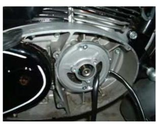
Remove the 3 fixing screws which hold the stator coil to its base. Now you can lift-off the coil a little away from the ground plate (ca. 1cm). So as the mounting holes on the ground plate become accessible. Don't damage the paint insulation!
