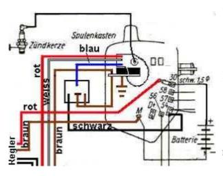
Connect the red, the white and the brown ground cable (from the new generator) and the blue cut-off cable to the new ignition coil.
