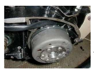
When the rotor is correctly installed, replace the spark plug. If you used the rear wheel to rotate the engine, change gears back to neutral.
