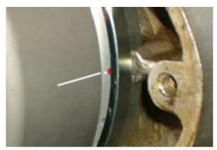
If you used the new rotor to turn the engine, carefully remove the rotor without changing the position of the crankshaft!
