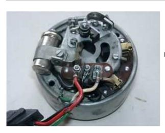
Losen all cables to the generator, regulator and ignition coil, then remove the generator with the regulator and ignition coil.
