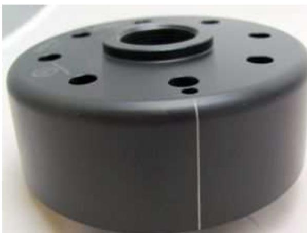
Have a look at the new rotor (flywheel). You will find on its circumference a small lasered on line. That is an ignition marking. It is durable, but not well visible, so better highlighten it with some marker pen.
