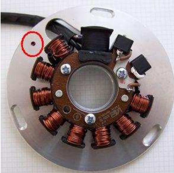
The base plate has - somewhat to the left of the wire opening - a small red dot which indicates the ignition marking.
