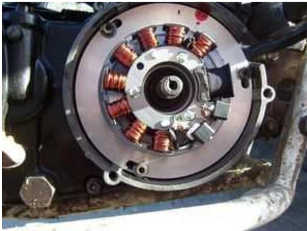
Place the new stator plate onto the engine and fasten there with the 3 screws M5 and the washer provided.
