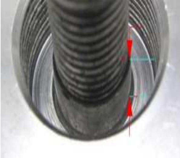
Further, you must check the end of the crank taper against the bottom surface of the puller hole of the rotor. With some engines the taper may be slightly above the bottom of the opening which will prevent the nut fastening the rotor securely if not detected and cured by adding a shim or in bad cases a distance piece. The rotor would slip in that case, making timing unsuitable.
