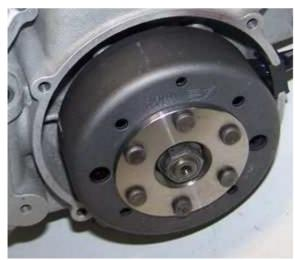
In that position, fasten the rotor carefully with the original nut.
