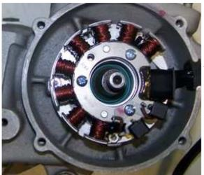
Put the stator coil back onto the plate, take care not the damage the wires. the stator has to snap in rather sharply. If it sets soft, you have probably jammed a wire underneath!
