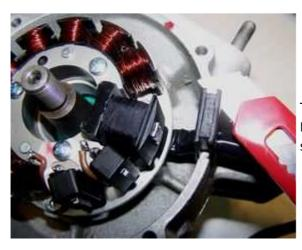
There is a rubber grommet on the stator wire. Press it into the wire exit opening and than cut the surplus material off carefully.
