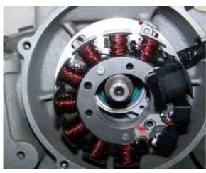
Unscrew the stator coil from the base plate and lift it a little away from it so that you can access the mounting holes. Take care not to damage the paint insulation of the coil.
