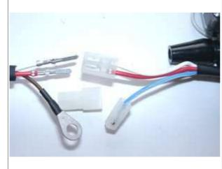
Look for the ignition coil with its female plug and the two wires (red and white).
