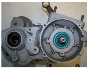
Unscrew the old stator and take it off the engine. Pull the rotor off, you will need a puller for this.
