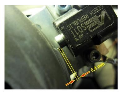
Put the rotor on but do not tighten it yet. Than turn the rotor slowly by hand and check clearance between the sensor and one of the rotor noses. This has to be ca. 0.4-0.5mm.
