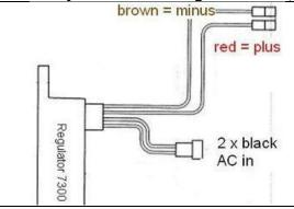
The new regulator/rectifier has 4 wires
