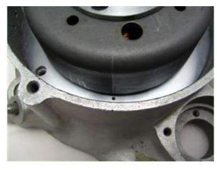
With shaft in TDC position, take the rotor carefully off again without changing the crank's position. Reset it onto the crank in such a way that the marking on the rotor aligns with the marking on the stator. If there is any change in the crank's position, you have to start again.
