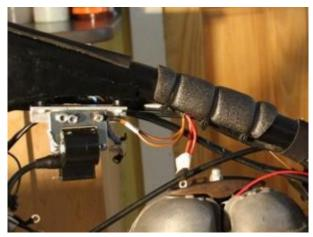
Fasten the new ignition coil beneath the tank. At some chassis is there a holder lug. If not, you can help yourself with <u>a self-made bracket</u> or wire binders.
