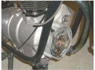
Unscrew the mounting screw that holds the armature on the crank shaft. It helps to engage the first gear, so you have stability. Take the three mounting stator screws off and pull the dynamo off. For this you will need the puller tool M8x90.
