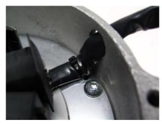
Then set the stator unit into the engine. Take care that the fixing holes of the case align with the holes of the stator unit. Screw it down with the 3 screws M6x20.
