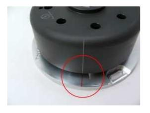
Rotor and base markings align in moment of ignition and are hence timing markings.
