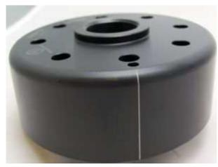
Have a look at the new rotor. You will find on its circumference a small lasered on (older rotor: pressed in) line. That is an ignition marking too. It is durable, but not well visible, so better highlighten it with some marker pen, preferably on top of the flywheel.
