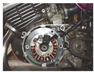
Put the new stator assembly into the place of your old magneto. Fasten the plate with the 2 screws M5. Don't use any other screws!
