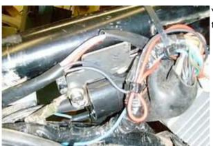
You will now have to fasten the ignition coil and the regulator to the frame of the motorcycle.
