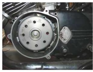
Take the rotor carefully off again without changing the crank's position and reset it onto the crank in such a way that the marking on the rotor aligns with the marking on the stator. In that position fasten the rotor carefully with the new rotor screw supplied.
