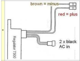
The new regulator/rectifier has 4 wires
