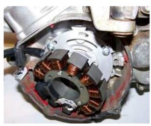
Place the new stator base onto the engine block. Fasten the plate with the base plate screws (please use the supplied ones, they need to be fairly flat).
