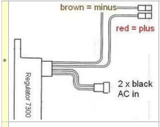
The new regulator/rectifier has 4 wires
