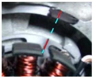
As this dot will not be visible any more once you have placed the rotor, you need to transpose the marking onto the outer casing as indicated in the picture below left.
