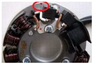
The base plate has - somewhat to the left of the 2 smaller black coils - a small red dot which indicates the ignition marking.
