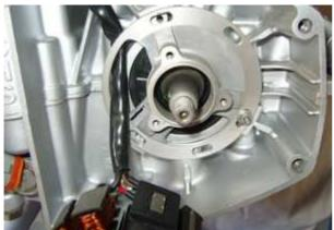
Unscrew the stator coil from the base plate and lift it a little away from it so that you can access the mounting holes. Take care not to damage the paint insulation of the coil.
