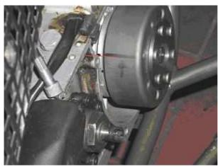
Take the spark plug out to ease turning of the crank and bring the piston into ignition position (put the rotor loosely onto the crank shaft and using it as a turning knob). Please consult your manual of the bike (125cm<sup>3</sup>: 0.7-1.2mm BTDC / 175-255cm<sup>3</sup>: 1.7-2.2mm BTDC).
