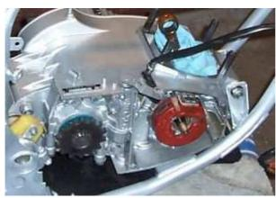
Disconnect the wires from the old dynamo. Pull all wires out of the engine housing.
