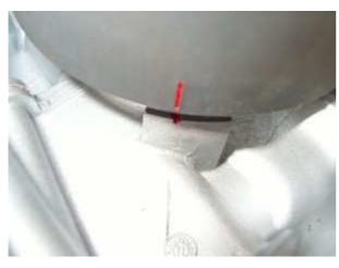
Take the rotor carefully off again without changing the crank's position and reset it onto the crank in such a way that the marking on the rotor aligns with the marking on the stator.
