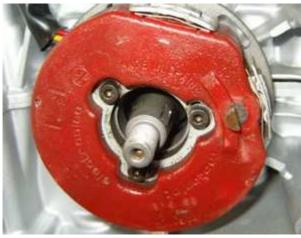
Loosen the nut on the rotor (with the appropriate tools) and pull it off with the help of the appropriate puller.
