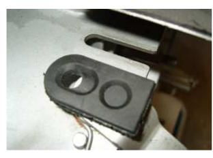
If you no longer have the original cable entry grommet and wanted to use the supplied, you must extend the designated slot on your engine. Make sure that it does not get chips in the oil seal.
