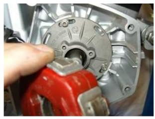
Loosen the 3 stator fastening screws and take off the Motoplat-unit. Then loosen the 3 screws on the base plate and remove the base plate.
