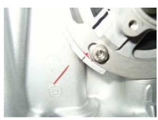
This ignition marking is no longer visible after the rotor is mounted. Therefore it must be later transferred to the motor housing.
