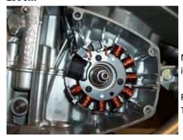
Magnet based generator with integrated solid state ignition. Output 12V/70W AC.
