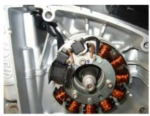
Put the stator coil back onto the plate, the bigger black coil shows about 10 o'clock. Take care not the damage the wires. the stator has to snap in rather sharply. If it sets soft, you have probably jammed a wire underneath!
