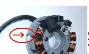
Have a look at the new stator. You will find on the circumference of its baseplate a small red marking. That to is an ignition marking.
