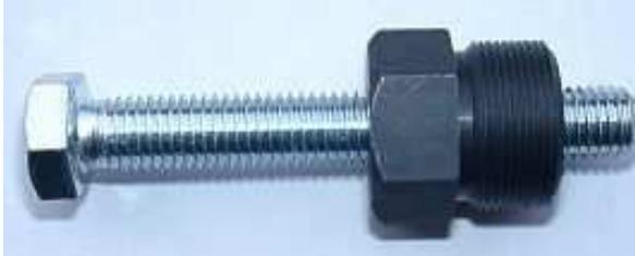
To pull the new rotor again, you will need a puller tool M27x1,25 (part 99 99 799 00 **-Not provided!-**).
