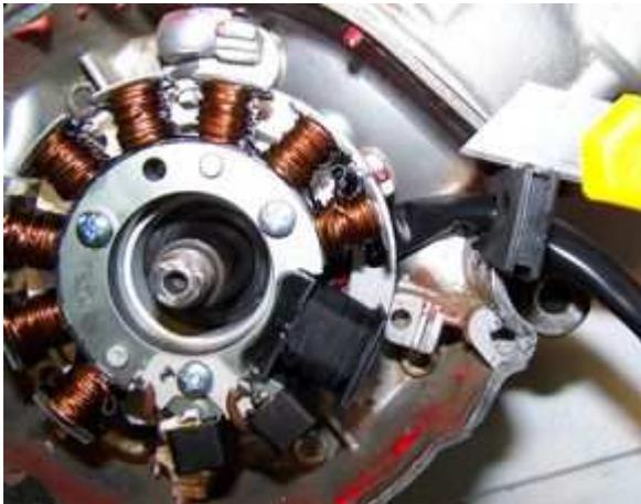
There is a rubber grommet on the stator wire. Press it into the wire exit opening and then cut the surplus material off carefully.
