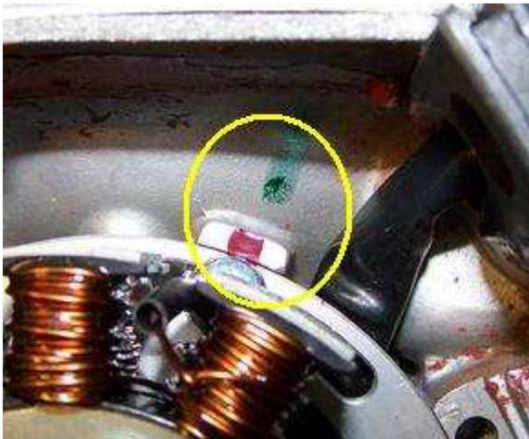
As the ignition marking on the base plate will not be visible once you have put the rotor, you will have to transpose it to some point further out. Already placing the holder screw there will cover the marking.
