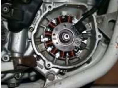
Magnet based generator with integrated solid state ignition, Light output 12V/70W AC. Ignition with own power supply from within the system. Replaces original Magneto as well as all ignition parts. Does not require changes on crankcase.
