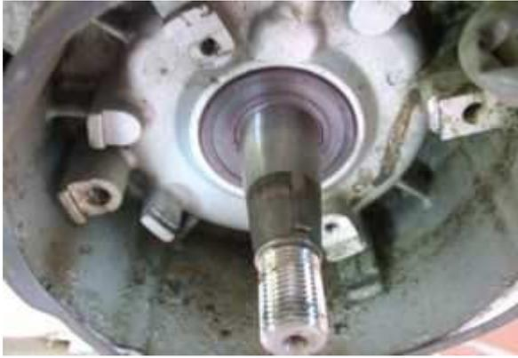
Pull the rotor off, you will need a puller for this. Unscrew the old stator and take it off the engine.
