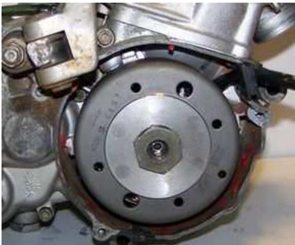
In that position, fasten the rotor carefully with the provided nut.
