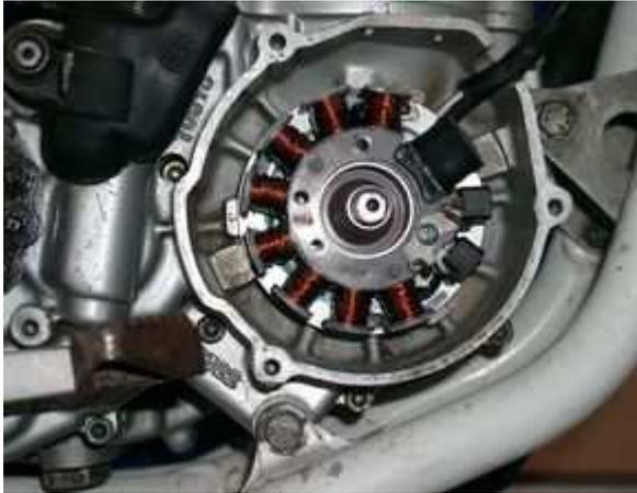
Put the stator coil back onto the plate, take care not to damage the wires. The stator has to snap in rather sharply. If it sets soft, you have probably jammed a wire underneath!
