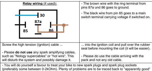
(even completely "brand-new") sparks plugs, terminals and cables. <u>- Do not use</u> spark plugs with an intern suppression resistor. NGK (e.g.) offered such spark plugs coded with an "R" (for resistor).
