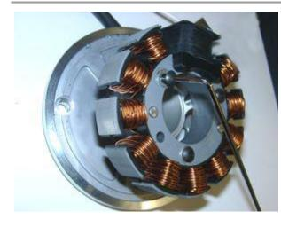
The new stator unit is pre-assembled, so that its construction is easier to recognise. For the mounting it has to be partly disassembled.
