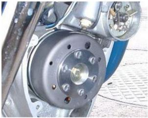
Place the rotor loosely onto the crank and check that it may move freely above the statorbase. Fasten the rotor carefully with the screw M7x40 (couter-clockwise tap). Please don't forget to use the washer.
