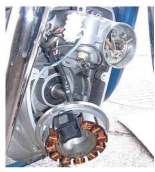
Put the pre-assembled stator plate (steel ring, aluminium plate and sensor) instead of the generator in the crank case. The sensor shows to the ground and the cable shows left up to the terminal of the ignition coil plate (if you look from the front on the unit).
