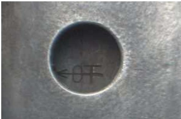
Take the spark plugs out. Place the rotor provisionally onto the crank shaft (without screwing it down there) for using it as a turning knob. Bring the crank shaft into TDC (in German OT) by using the spyhole.
