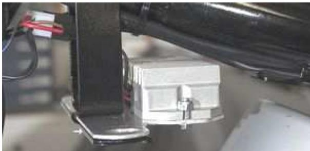
The new regulator/rectifier could be fitted under the rear holder for the petrol tank. (On this proposal the customer has used a self made [unit plate](#).) For this, unscrew the nut (spanner 13) securing your BMW's tank holder and put your new regulator plate (with the regulator on it) underneath. The regulators cooling fins will face upwards. Put the nut back, do not forget to put the washer back.
