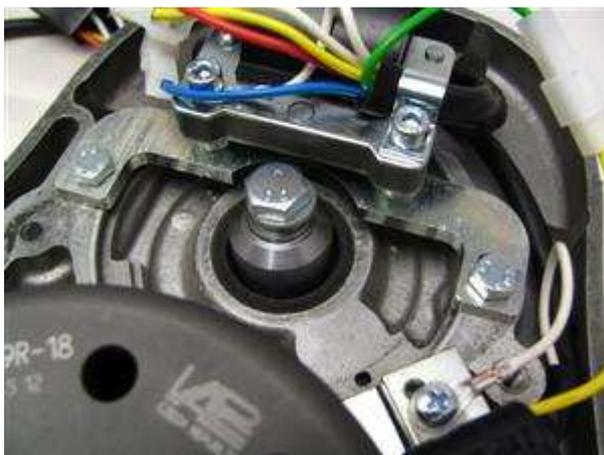
Place the provided oil-seal cam onto the camshaft and fasten it with the special screw M8x40. Please don't forget to use the provided washer.
