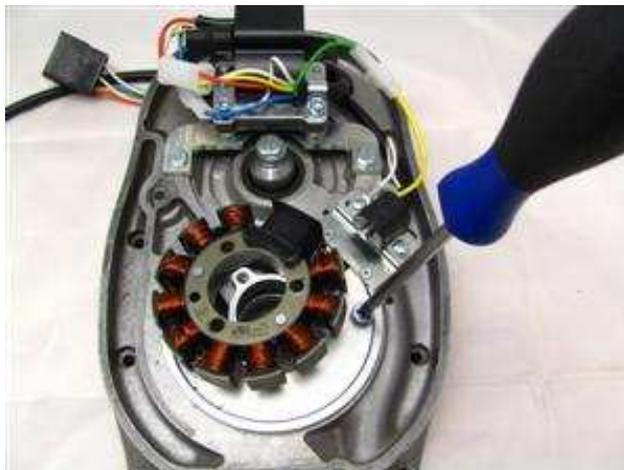
The new stator unit is pre-assembled so that you can recognize its structure more easily. To install it, it has to be partially disassembled however. Take care not to damage the paint insulation of the coils. Unscrew the new stator coil from its base plate (the 3 hex screws) and lift it a little away from it so that you can access the mounting holes in the base plate.
