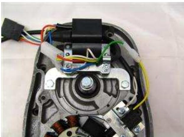
Screw the 2 high tension cables (if supplied as one, cut it into 2) into the ignition coil.
