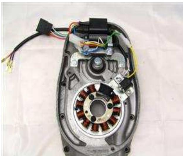
Now put the stator coil back into its position on the plate, taking care not to damage the wires. Make sure that the inner opening of the stator unit slots evenly over the elevated fixing rim of the base plate - otherwise the coil will sit loop sided and will touch the rotor, damaging it.
