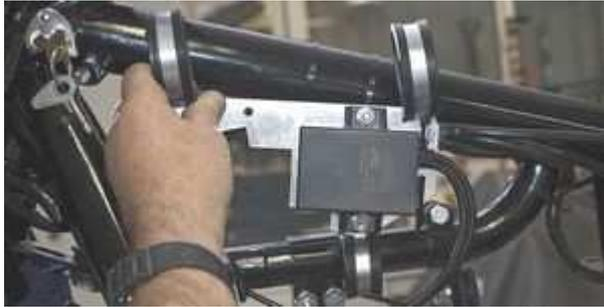
The supplied mounting plate for the new advance unit and the attached clamps do not fit on any BMW frame. It must be modified or replaced in individual cases.
