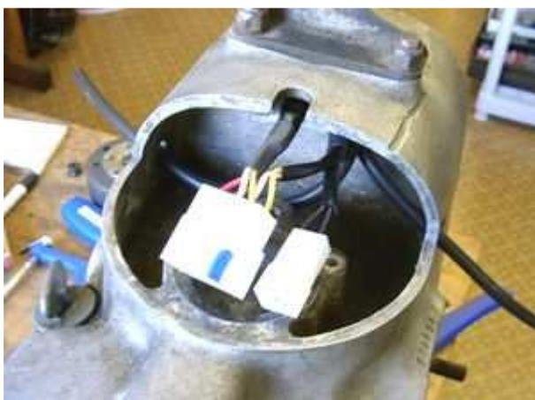
The short harness pieces running from the new generator und the coil unit will be ushered with theirs plug-ends through the top opening into the rear top engine compartment. They wait there to get connected to the rest of the assembly.
