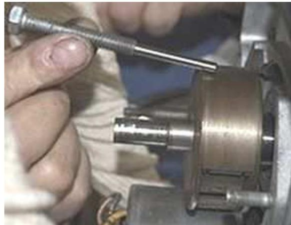
Now remove the 2 nuts (spanner 10) which hold the magnet unit and take the part off the engine casing. Use again the hex key 6mm and remove the screw that retains the rotor on the nose of the crankshaft. In place of the now removed holder screw install the BMW rotor puller and screw it in till the rotor pops off (again, you will have to hold the rotor with your hand, and you might well have to use a
