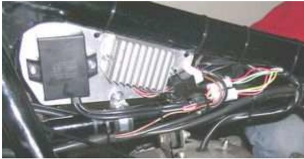
As this picture shows, it is also possible to mount the regulator on the advance plate. This will depend on specific frame configuration.
