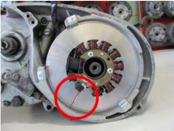
Have a look at the stator base. You will find near the top left fastening hole a small red marking on the baseplate. This is an ignition marking.
