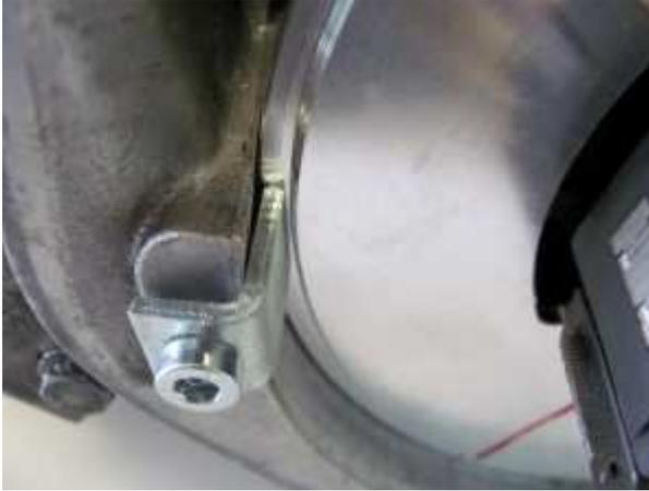
Nox arrest the plate by help of the 3 holder clamps.
