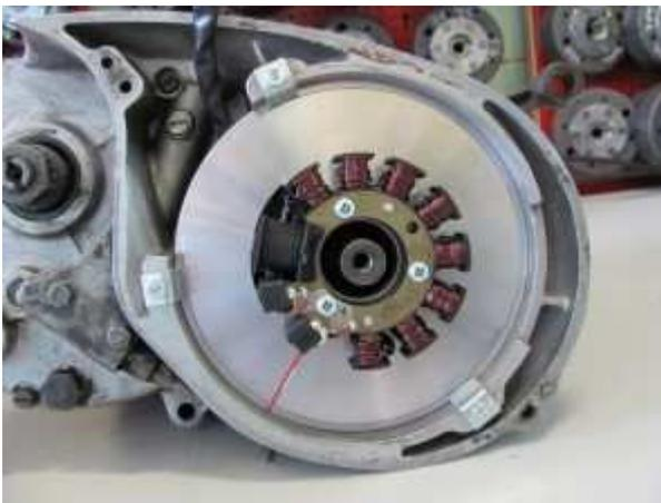
Place the new stator unit into the place of your old dynamo.
