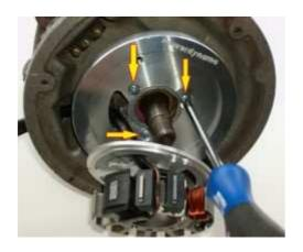
Put the adapter plate (with the stator hanging loosely from the unit) into the place of your old generator. Fasten the plate with the 3 screws M4x35 provided.
