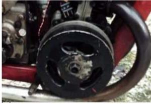
Remove the original JAWA rotor and the stator coil.
