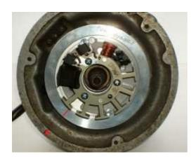
Once the plate is fixed, reset the stator coil onto it. Here make double sure not to pinch any wires underneath. As the coil sits quite low in the engine, this is difficult to see.
