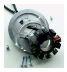
At first loose the three fastening screws of the stator and lift it carefully from its base plate. At next unscrew this base plate from the adapterplate. Keep in mind how the two plates were screwed together.
