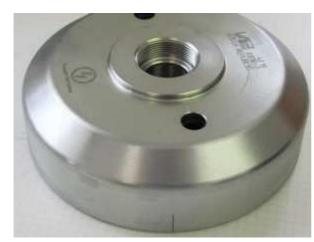
Have a look at the new rotor. You will find on its circumference a small pressed in line. That is an ignition marking. It is durable, but not well visible, so better highlighten it with some marker pen.
