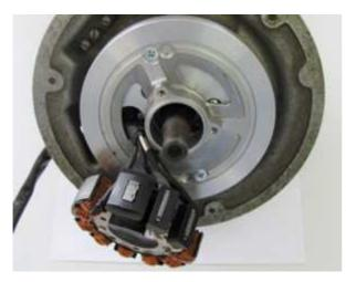
Now place the stator ground plate onto the adapter plate and screw it down with the both countersunk screws M5x10.
