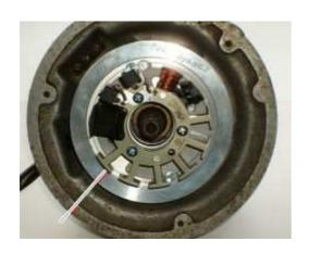
The ignition marking on the adapter plate will be hidden by the rotor. That is why you have to prolong the marking on the engine case.
