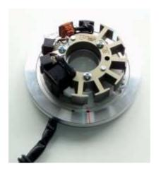
Take a look at the new stator unit. Near the cable exit you will find a small red ignition marking.
