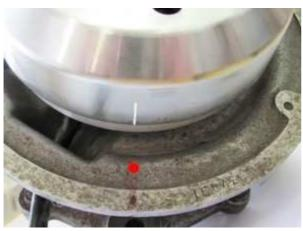
Take the spark plug out to ease turning of the crank and bring the piston into ignition position (put the rotor loosely onto the crank shaft and using it as a turning knob). Please consult your manual of the bike (eventually 6mm BTDC).
