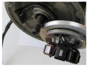
Now take this apart bolted stator unit and run the cable out through the output of the motor housing.
