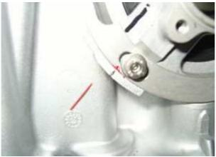
This ignition marking is no longer visible after the rotor is mounted. Therefore it must be transferred to the motor housing.
