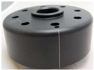
Have a look at the new rotor. You will find on its circumference a small lasered in line. That is an ignition marking. It is durable, but not well visible, so better highlighten it with some marker pen.
