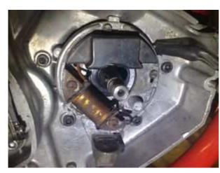
Disconnect the wires from the old magneto Pull all wires out of the engine housing. Remove all cables which go to the old ignition coil,take the ignition coil off.
