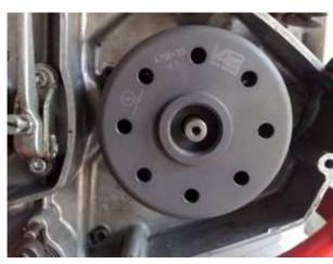
Take the spark plug out to ease turning of the crank and bring the piston into ignition position (put the rotor loosely onto the crank shaft and using it as a turning knob). Please consult your manual for the needed ignition value (if you do not find anything try 2mm BTDC).
