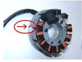
Have a look at the new stator. You will find on the circumference of its baseplate a small red marking. That too is an ignition marking.
