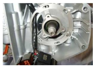
Unscrew the new stator coil from the base plate and lift it a little away from it so that you can access the mounting holes. Take care not to damage the paint insulation of the coil.
