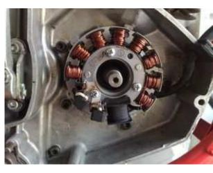
Put the stator coil back onto the plate, the black coils showing into wire exit direction. Take care not the damage the wires. the stator has to snap in rather sharply. If it sets softly, you have probably jammed a wire underneath!
