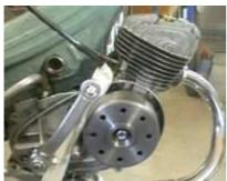
Magnet based generator with integrated, maintenance-free solid state ignition. Output 12V/70W AC. There is no need for changes on engine casing.
