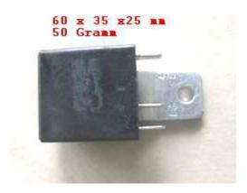
Fasten the new AC-regulator at a convenient place too, maybe beneath the seat or the side casings.
