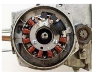
Put the base plate with the stator hanging loosely from the unit into the place of your old generator. Fasten the plate with the 3 screws M4. Take care to not jam any wires under the plate.
