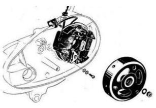
Remove all cables from the old generator and ignition coil and take off these parts.
