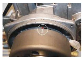
Take the spark plug out and bring the piston into ignition position. Might be 2mm BTDC.
