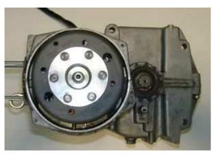
Take the rotor carefully off again without changing the crank's position and reset it onto the crank in such a way that the marking on the rotor aligns with the marking on the stator. In that position fasten the rotor carefully with the original nut.
