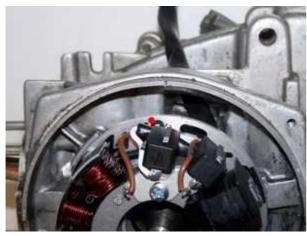
The ignition mark of the stator is not visible after the rotor was put onto the crank shaft. You have to transfer the marking to the engine body.
