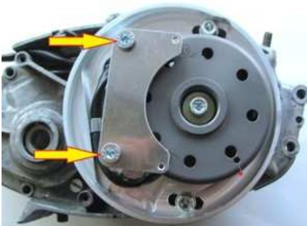
Replace now the cover holder plate on the ground plate. You have to put the two M8x60 screws through the holes in the cover holder plate and the two spacers. Then screw it tight on the ground plate.
