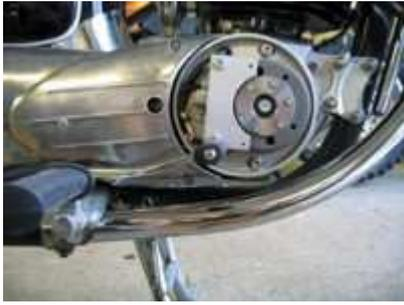
Magnet based generator with integrated fully electronic ignition. Output at 12V/100W DC. Solid state electronic ignition with own power supply from within the system. Replaces [old 6V Noris dynamo of type MLZ](#) including ignition coil and controller. You may [drive without a battery](#), if you want and if you following some advices. No changes on engine casing needed.
