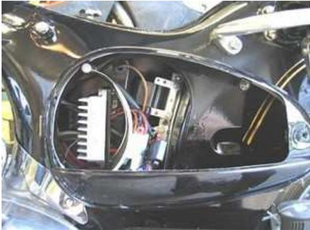
Fasten the regulator/rectifier unit, the relay and the ignition coil on a convenient place, maybe in the side pocket.
