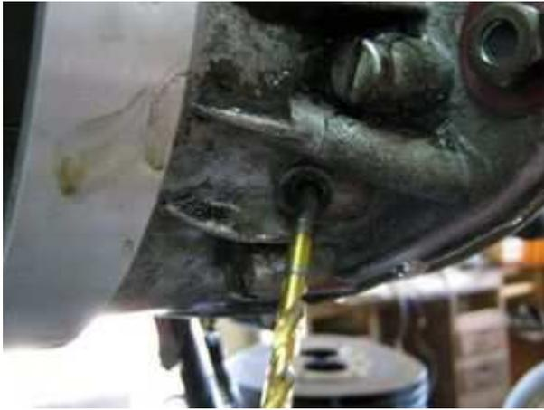
Introduce (carefully) a 3mm dia and 100 long metal pin (say a drill 3mm with its non spiraled end) into the timing opening.
