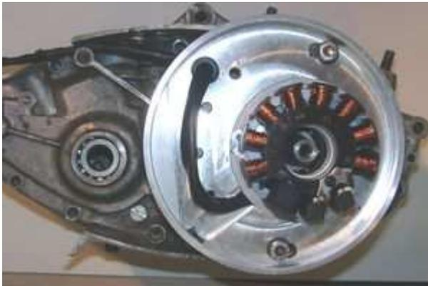
Take off the cover holder plate from your new generator. Place the preassembled unit (ground plate/stator) at the ignition system mounting of the crank case. Screw it tight with both M8 screws. You should set the screws in the center of mounting holes, so you have the possibility for correction. Please don't forget to use the washers.
