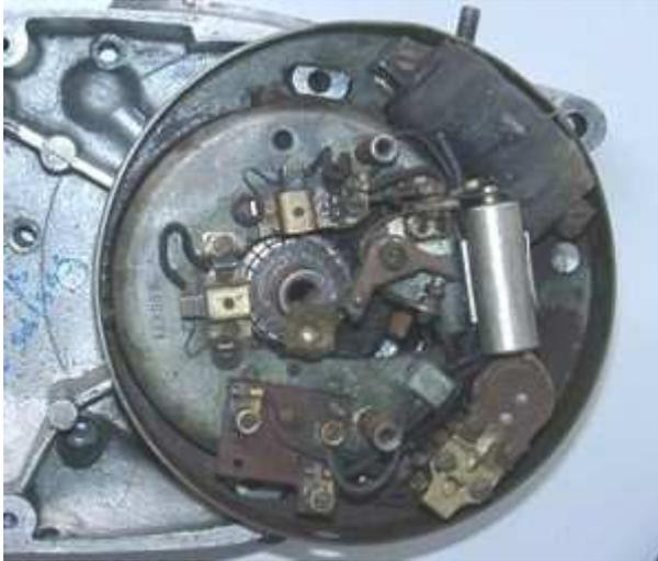
Disconnect the cables from your old generator and remove it. Unscrew the old stator and take it off the engine. Pull the rotor off, you will need a puller screw for this.
