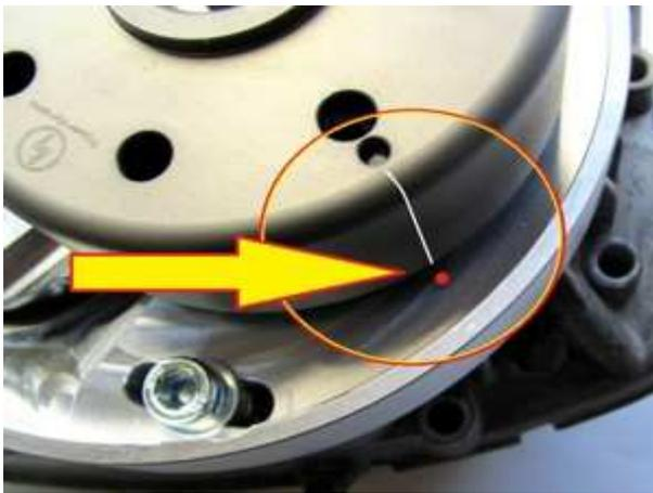
Have a look at the new rotor. You will find on its circumference a small pressed in line. Then have a look at the ground plate. There you will find a red point marker. These are ignition markings. They have to align at the point of ignition.
