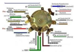
Wiring of the ignition lock for the new system.
