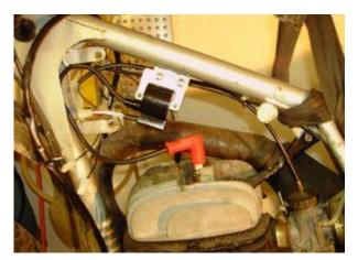
Fasten the ignition coil on the frame of the motorcycle, best there, where the original coil was.
