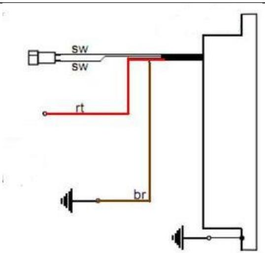
**- The regulator of this system:** has a inbuilt smooting condenser which enables full function of flashers and horn with or without a battery present:
