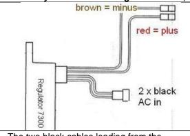
The new regulator/rectifier has 4 wires
