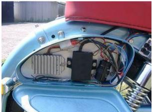
Fasten the new regulator/rectifier and the advance unit ("Black Box") at a convenient place, maybe in the side case (or any disired place).
