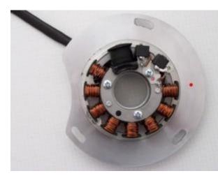
Have a look at the new ground plate (with the stator). You will find there a red marking. This is an ignition marking.
