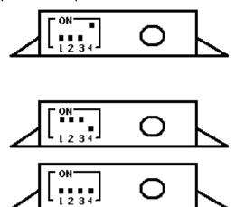
The most suitable curve for the Max will be activated by setting switch 4 to ON and switches 1/2/3 to OFF (against ON). The engine will reach full advance of 40° at 3.800rpm. Revolution throtteling from 8.500rpm.
