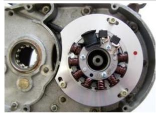
Screw down the new stator unit with the 3 screws M6 to the crank case. Don't forget to use the washers.
