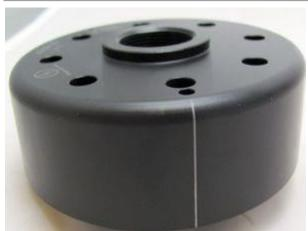
Have a look at the new rotor. You will find on its circumference a small pressed in line. That is an ignition marking too. It is durable, but not well visible, so better highlighten it with some marker pen.
