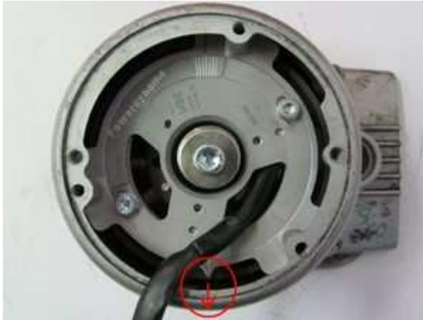
Place the cover with the fitted new stator into the engine.
