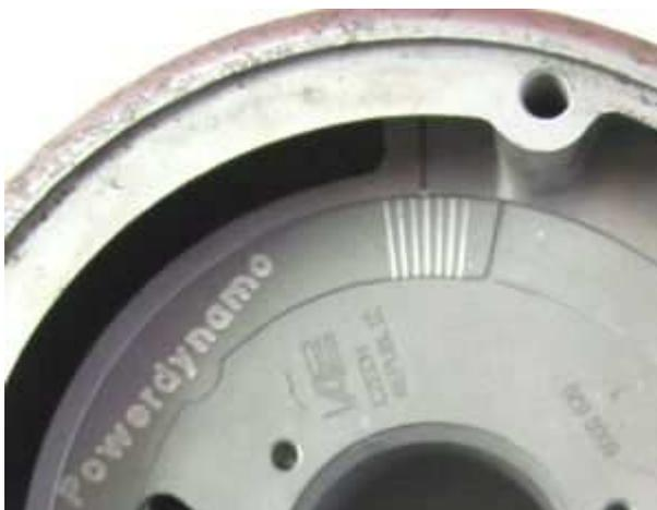
Now, to fine tune, you may loosen **a little (!)** the 2 holder screws you have at the bottom and turn the base (magnets will pull against you) until the 2 markings align.
