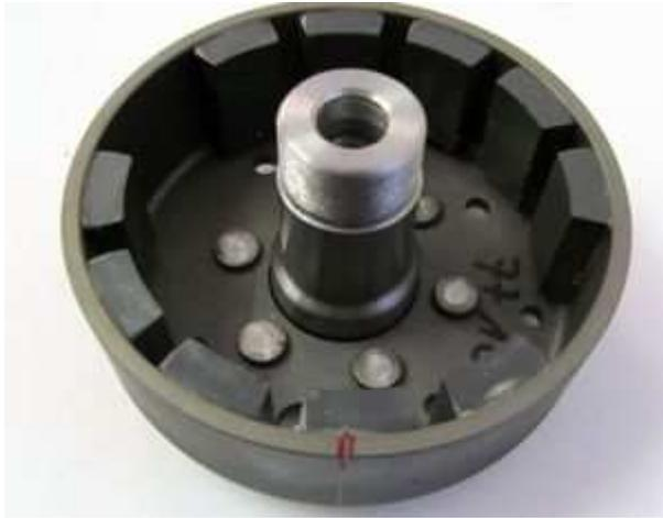
Check the inside of the rotor for foreign objects (screws or other metal parts) that could damage the rotor and stator during the operation and - without having changed the crank position which should be set as shown above - place the rotor in such a way on the crankshaft (the open side with the view at the magnets facing you) that the marking is about vertical to ground (facing downwards).
