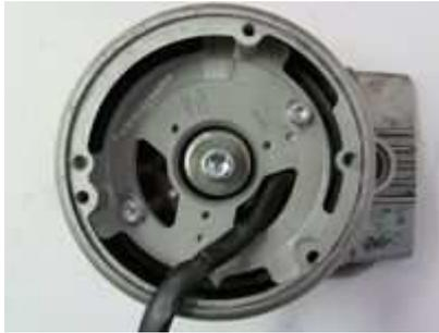
generator/electronic ignition for [Suzuki T125](#) (not for GT125!)
