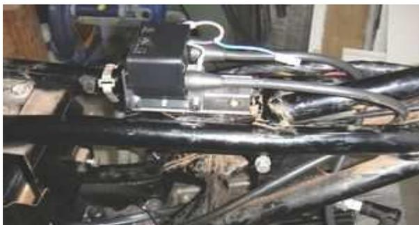
Fasten the new electronic rectifier/regulator and ignition coil at a convenient place. Before you fix the coil, screw in the high-tension cables. Lay the new generator cables along the frame (using the enclosed cable binders), in that way, that they finished close to the regulator resp. ignition coil. Take care that nothing's pinched.
