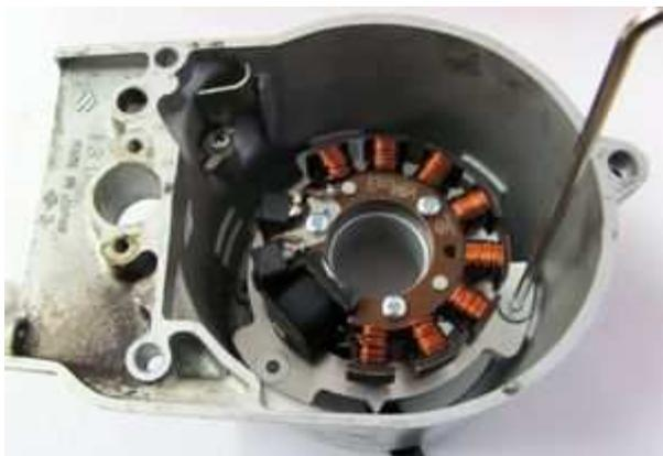
Place the new stator unit into the engine cover as shown here. Fasten with the 3 countersunk screws M6 provided.
