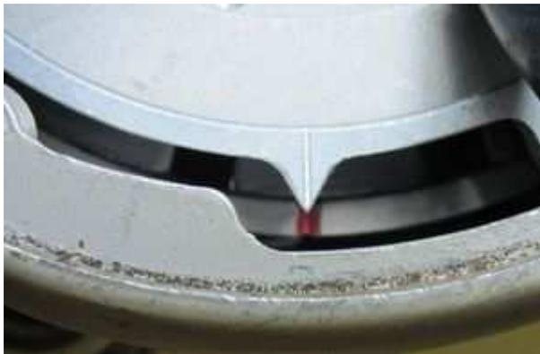
With crank still in ignition position check whether the rotor marking and the stator indicating pin align.
