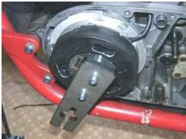
The same tool can be used to pull the rotor off again.
