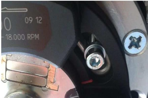
To be able to make use of the long holes to modify timing, set the screws into the middle position of those oblong holes.
