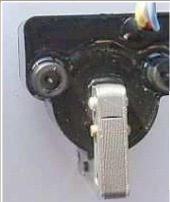
In our twin outlet coils both ends of the secondary go to spark plugs.
