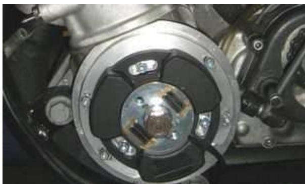
Place the adapter onto the engine. The wire opening of the adapter will show towards wire exit. Screw the adapter down with the 4 supplied screws M4x16.
