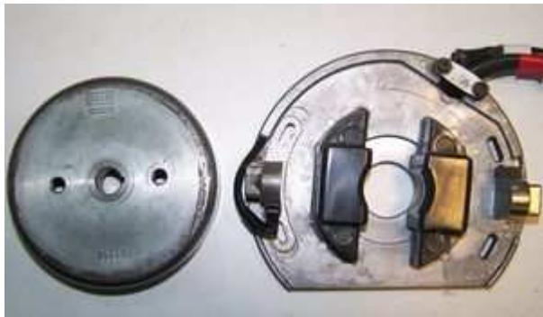
Take the old ignition system (including ignition coils) off. Take the woodruf key or arresting pin from the crankpin (so you have there).
