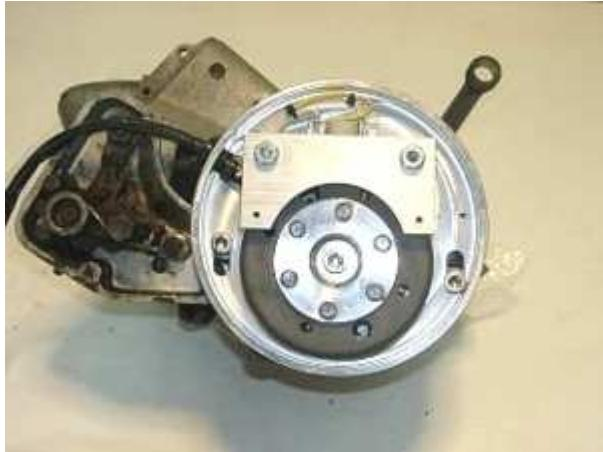
Replace now the cover holder plate on the ground plate. You have to put the two M8x60 screws through the holes in the cover holder plate and the two spacers. (The upper side of the plate is marked by a small bored hole!) Then screw it tight on the ground plate.
