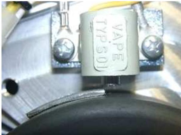
Pull the rotor carefully off the crank (without changing the crank's position) and reset it again so that the sensor's right edge aligns to the left edge of the sensor core. Take care that during this procedure the crank doesn't move, otherwise you have to start again. In this position (see left) tighten the rotor by the screw M8x50, not forgetting the supplied washer.
