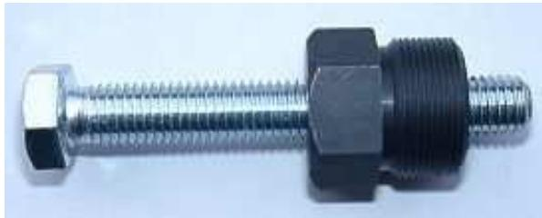
To pull the new rotor again, you need a puller screw M27x1,25 (part 99 99 799 00 **-not provided-**).
