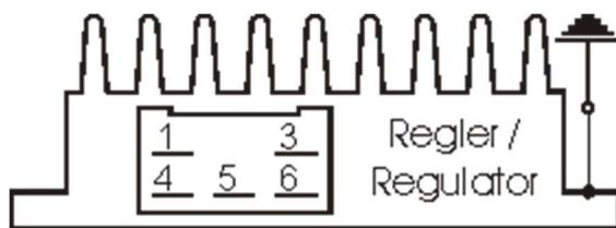
The new regulator/rectifier has a compact plug with 6 positions, of which one is not used. A female plug cover fitting to this plug is delivered. Into this female plug you have to insert the following wires (which have terminals that snap into the plug):
