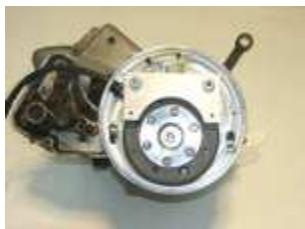
Magnet based generator with integrated fully electronic ignition.
