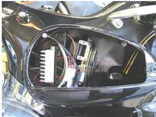
Fasten the regulator/rectifier, the relais and the ignition coil at a convenient place.
