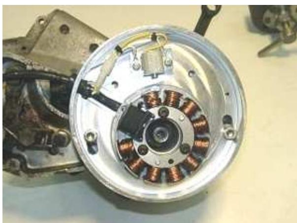
Take the preassembled cover holding plate off the new generator. Put the ground plate/stator unit onto the crank case and screw it down with the 2 screws M8. Don't forget to use the washers.
