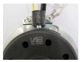
With the crank in ignition position, pull the rotor off again carefully - make sure that by doing this, you will not alter the crank position - and set the rotor again back onto the crank in such a way that the left edge of one (any of the two) of its noses aligns with the right edge of the sensor pin (that is when the nose just reaches the sensor pin).
