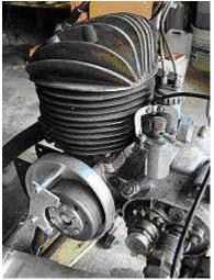
Magnet based generator with integrated solid state ignition Output at 12V/100W DC.
