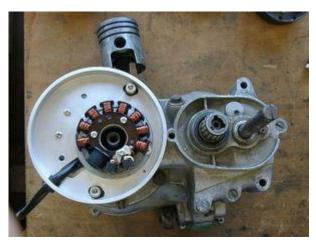
Take the preassembled cover holding plate off the new generator. Put the ground plate/stator unit onto the crank case and screw it down with the 2 screws M8. Don't forget to use the washers.
