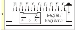
The new regulator/rectifier has a compact plug with 6 positions, of which <u>one</u> is not used. A female plug cover fitting to this plug is delivered. Into this female plug you have to insert the following wires (which have terminals that snap into the plug):
