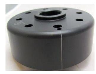
Take a look at the new rotor. You will find on its circumference a small pressed-in line, an ignition marking too. Both aligns at the point of ignition.
